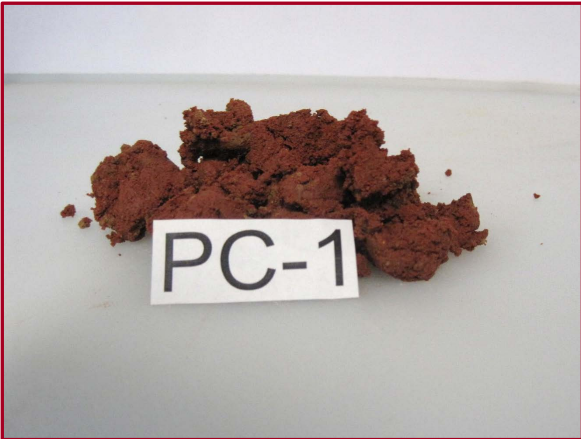
FIGURE 5C: PHOTOGRAPH OF SAND-CLAY BASE (LBR 75) ENCOUNTERED AT PAVEMENT CORE PC-1
