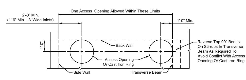
Only one access opening is allowed in each segment of inlet top between an outside wall and a transverse beam or between two transverse beams.
