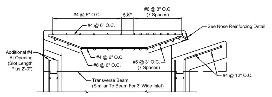
PARTIAL SECTION - 4'-0" THROUGH 6'-0" INLET WIDTH (Section Of Inlet With Slot)
