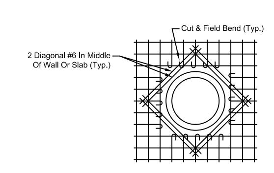
REINFORCEMENT AT WALL OPENINGS
