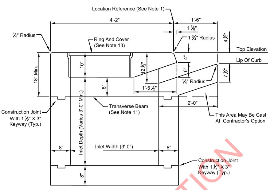
SECTION GG - 3' WIDE INLET (Optional Opening In Bottom Slab Not Shown)
