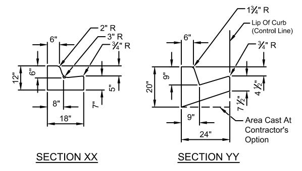
**GUTTER TRANSITION FOR USE** WITH 18" CURB & GUTTER
