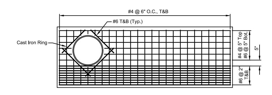
TOP SLAB REINFORCEMENT PLAN - 3' WIDE INLET
