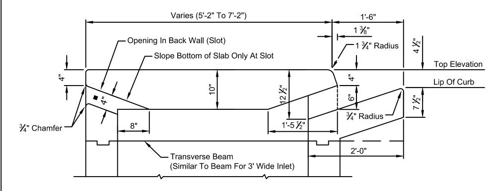
PARTIAL SECTION - 4'-0" THROUGH 6'-0" INLET WIDTH (Section Of Inlet With Slot)
